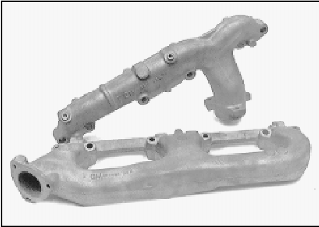
The Stock Manifolds And Mufflers selection assumes that the exhaust manifolds are a typical, production, cast-iron “log-type” design, where all ports connect at nearly right angles to a common “log” passage.
