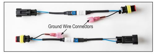
Do not connect the ground wire to the positive battery terminal. Doing so could cause damage to the ECM or the VIED.
